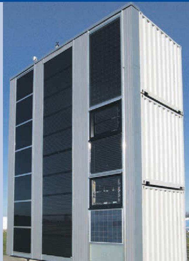
Fig. 1 – Test façade for various building integrated PV systems (Photo: Maria Roos, Fraunhofer IWES, Kassel).
