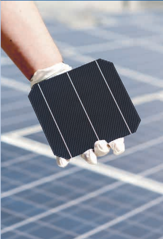
Fig. 2 - In January 2015, IMEC demonstrated a large area industrial crystalline silicon n-PERT solar cell with a record 22 percent efficiency.
