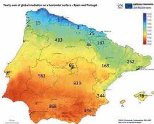
Fig.5 - PV power (MW) installed per autonomous community as of December 2013 (Source: CNE-UNEF).
