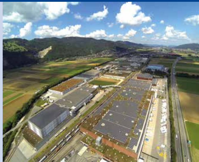
Fig. 4 - Migros Logistics Centre, Neuendorf, Switzerland. 5.2 MW on-roof PV system (Photo: Tritec AG).
