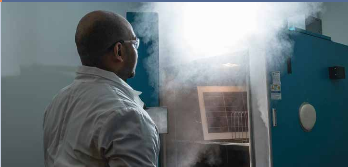
Fig. 3 - Alliston Watts removes a PV module after a damp test for accelerated stress testing (Photo: Lindsey Dillon).
