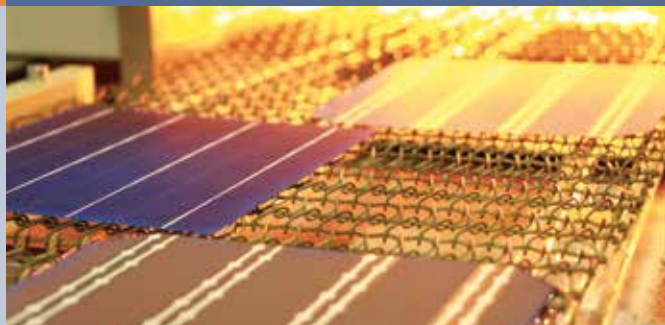
Fig. 4 - mc-PERC and ZEBRA-solar cell at the exit of an annealing furnace (Photo: © RCT Solutions and ISC Konstanz).
