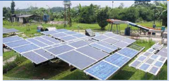
Fig. 3 - PV module reliability test site in Indonesia studying the stress factors of PV modules failures under real time outdoor testing compared to accelerated stress conditions (Photo: TÜV Rheinland).
